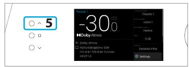
6. Select the Network item and press the Volume knob to validate. This will give access to the Network info where you can take note of the IP address and also reset the network parameters when needed. Select Back to exit.
